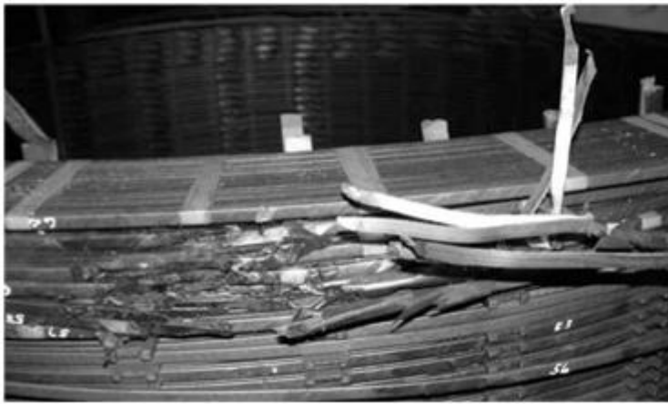
Fig. 2. Windings of Eskom transformers presumed damaged by the geomagnetic storm on 29 October 2003.
